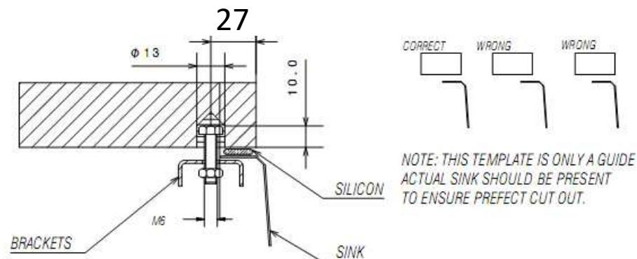
2) Determine placement of clip brackets. Pre-drill holes according to method desired based on countertop material.
